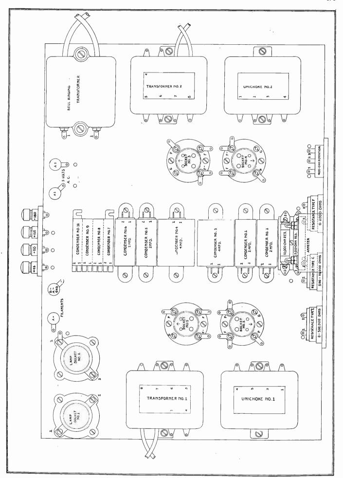
two unichokes, the filter and by-pass condensers, the bell ringing transformer, four UX sockets, two porcelain Mazda bulb sockets, four binding posts, a double resistor mount and a binding post strip. Before mounting any of the parts, draw a pencil line on the board parallel to the 12-in. edges, dividing it into two equal parts.
