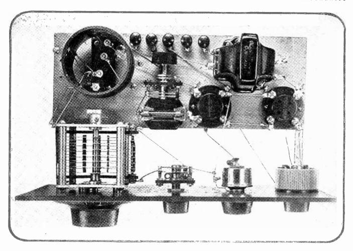
turns for the grid coil and three turns for the tickler. Similarly, for the 30 to 45-meter band, use seven turns for the grid coil and five turns for the tickler. To reach up to 100 meters use No. 22 wire with nineteen turns for the grid coil, and six turns for the tickler.
