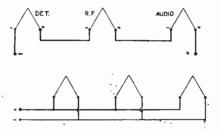
Fig. 1. Below: Parallel filaments. Fig. 2. Above: The new series method.
