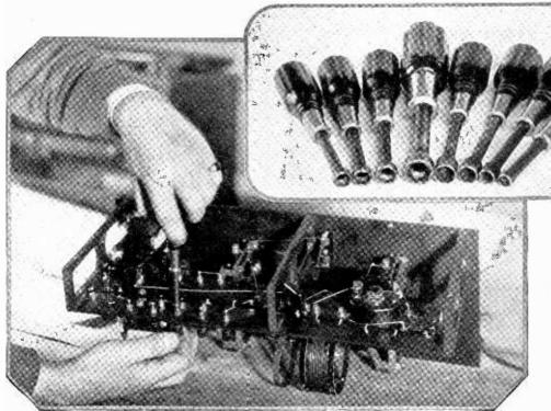
Some of the different sizes of round and hexagonal Spintites, and an illustration of their use. Much more positive connections can be made with Spintites than with pliers, because the Spintites grash the round or hex nuts in a firm grip
