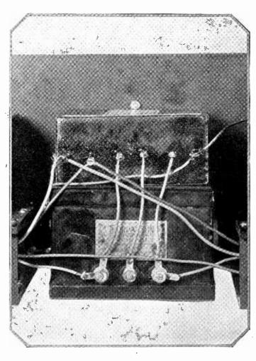
a loudspeaker will work better connected one way rather than another, but if you reverse the connections of the speaker to the output transformer, no difference will be noticed. This is due to the fact that no direct current flows through the speaker and therefore there is no tendency for any current to magnetize or demagnetize the speaker magnet, another decided advantage of the output transformer.
