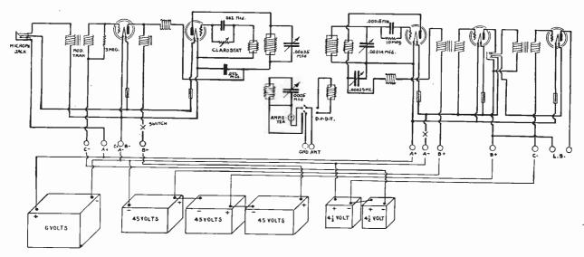
Complete hook-up for B battery operated short wave telephone transmitter and receiver
